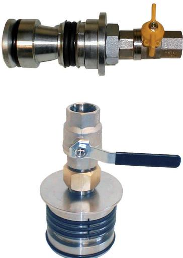
Pressure Test Ends were designed to provide a simple mechanical means to facilitate pressure testing of PE pipe installations either with pressurised fluid or gas. All sizes listed are designed to withstand an internal pressure of 12 bar and small sizes up to 125mm have been found to be pressure tight to the burst pressure of the pipe (over 40 bar).
